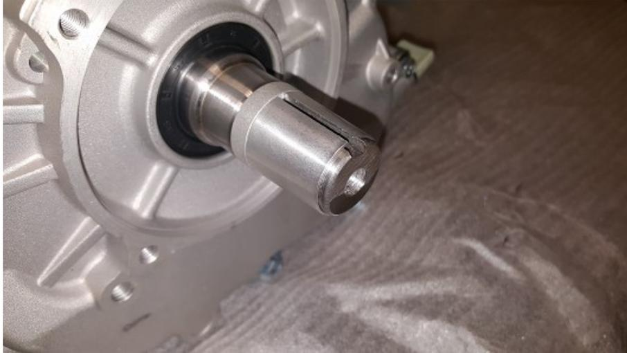
3. Assuming you are keeping the 3/8-24 thread, you will need to drill & tap the threads deeper. Carefully drill an additional 3/4" into the crankshaft using an "S" drill bit. Clean the hole with compressed air to ensure its clear of chips.
