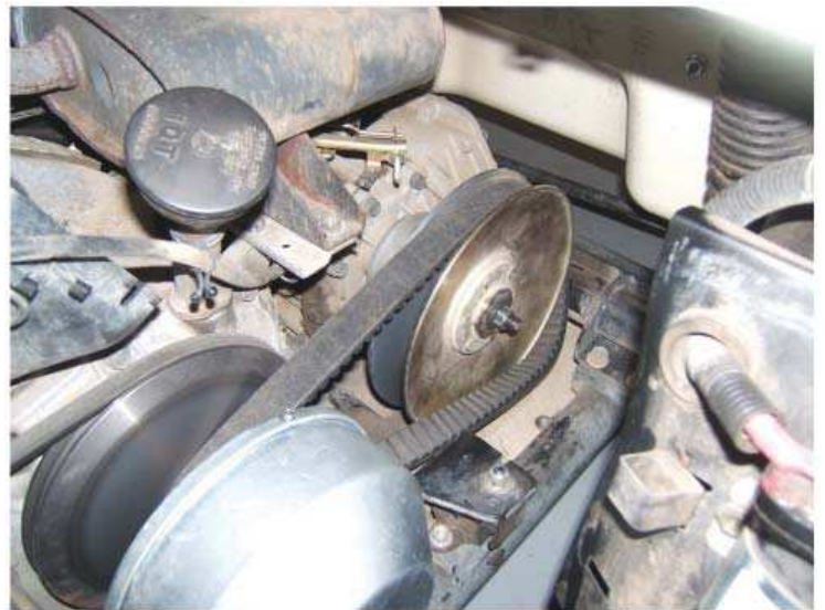
Position the belt as shown and rotate the driven clutch clockwise
